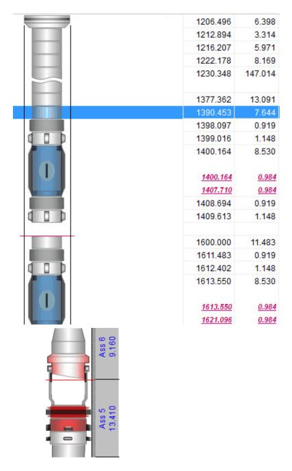
Fig. 1: The second pup joint has been set to Fixed Depth = 1600 m Stem is stung into a PBR by setting the PBR to a fixed depht
