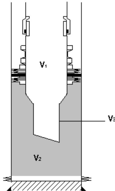
The volume down to the perforations is given by  $V_1 + V_2 - V_3$
