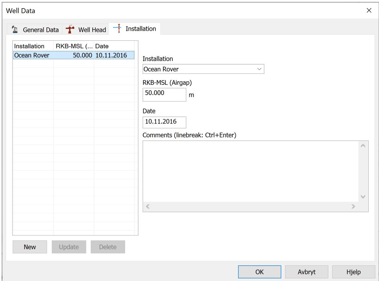
Press the New button and choose a rig from the Installation dropdown. Enter the correct RKB-MSL (Airgap) and press Update. The set Installation and airgap will now be the new datum.
