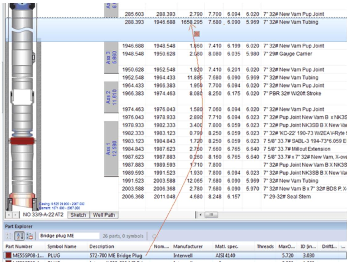
You will now see the plug inside the tubing, but to adjust the depth right click on the tubing
