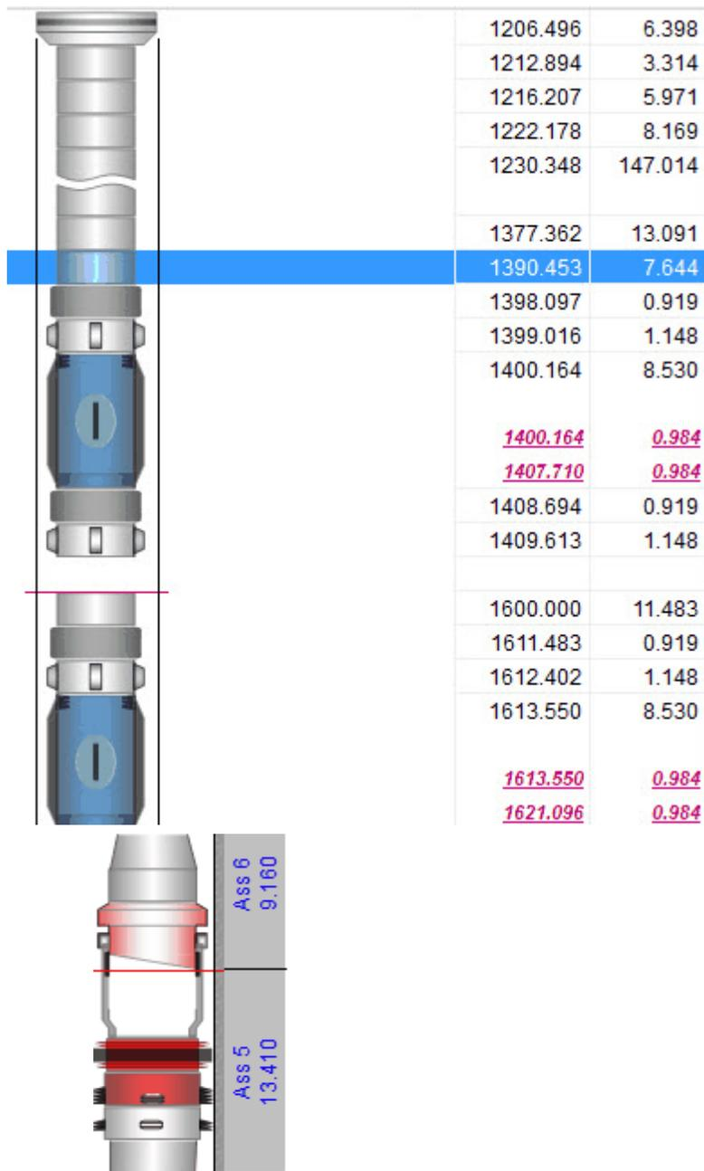
Fig. 1: The second pup joint has been set to Fixed Depth = 1600 m
