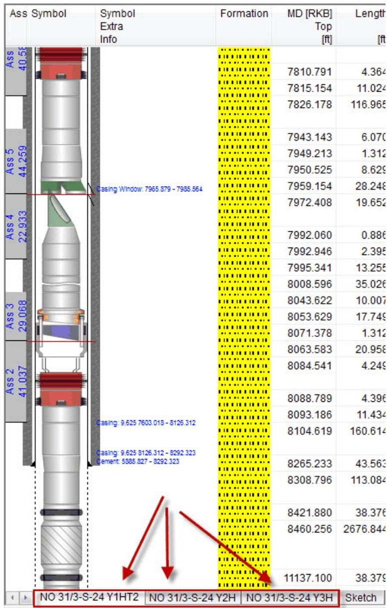
A lateral bore should start with the first element attached to the cross-section of the parent wellbore, or from the hanger section inside the parent wellbore.
