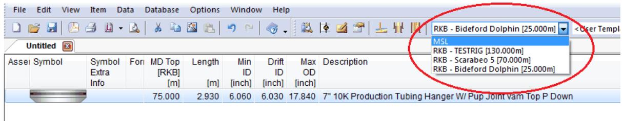
When you have set datum and are ready to start building the string, you have to enter the MSL-Tubing Hanger (Landing point / shoulder) depth in the [General Data](#) tab in the Well Data dialog. This value is set for CSD to calculate the correct RKB-Tubing Hanger depth, which will be the top depth for the first element in the completion schematic. If you don't have the MSL-Tubing Hanger depth, you can use the following equation to find it:
