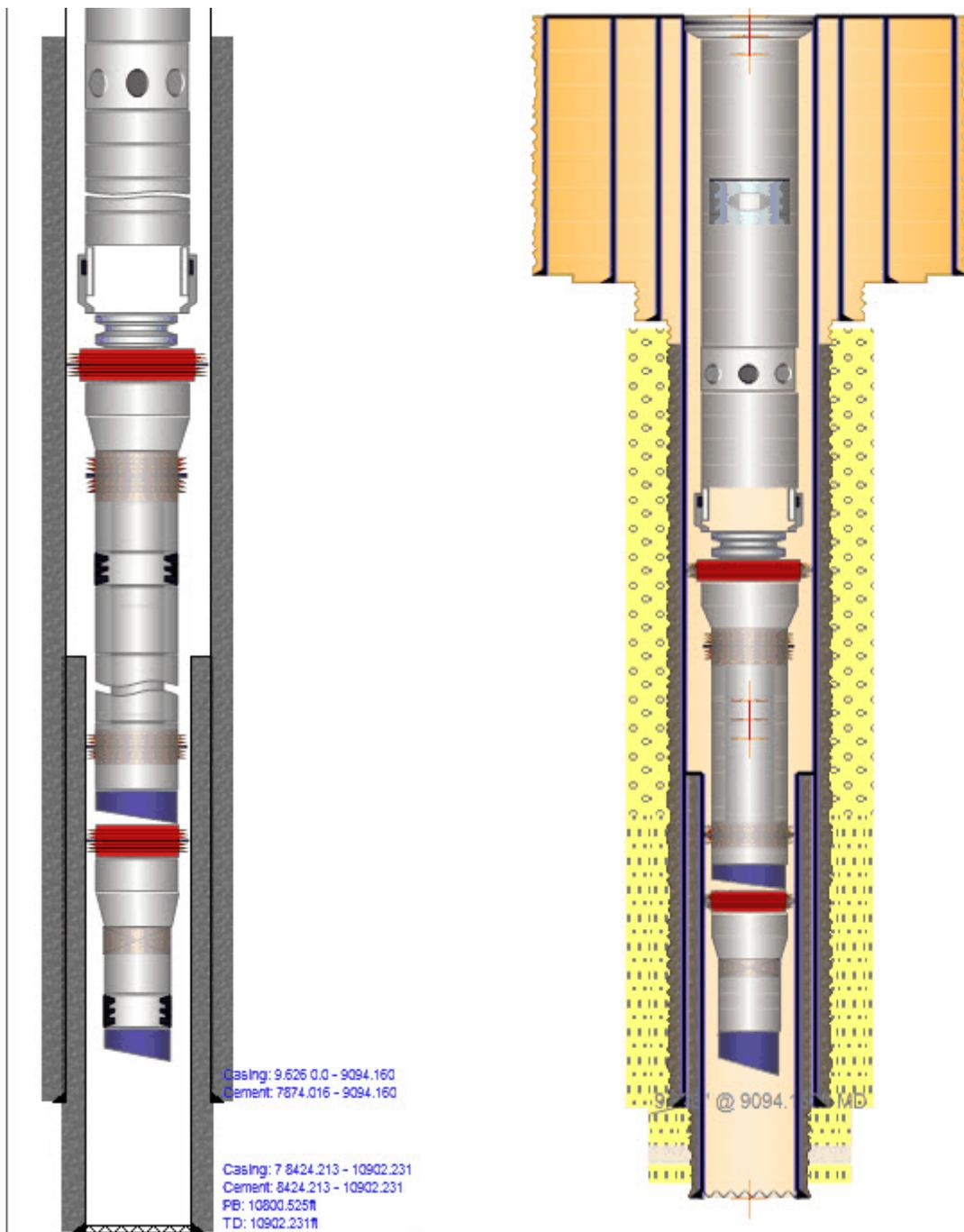
**NOTE:** In Schematic mode, you can view the cement for the inner casings only. Go to the Sketch mode to view the cement for all casings.
